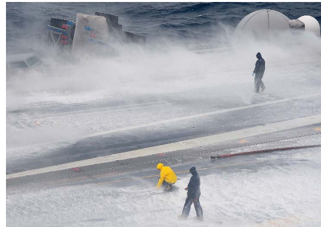
Fire Drill using AFFF
